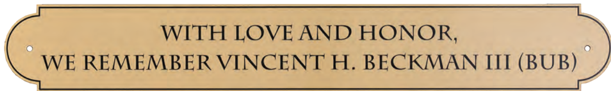
▲ 2-1/4" H x 15"W Etched and color-filled .040" brass, laser cut shape with two corner holes-1/8" dia. placed 1/8" center to edge
